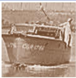
In 1947, the U.S. Coast Guard built 40-foot patrol boats using fiberglass composite materials. These boats were used until the early 1970s, when they were taken out of service because the design was outdated. After the boats were decommissioned, the composites were thoroughly tested and found to have lost only 2 to 3 percent of their original strength during 25 years of hard service.
