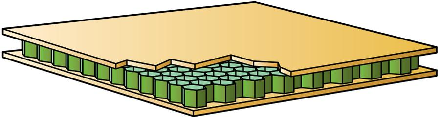
**Honeycomb** is a core material made from sheets of resin-soaked material shaped into cells (openings) like those of a beehive's honeycomb. This structural material is strong, lightweight, and used in sandwich construction.
