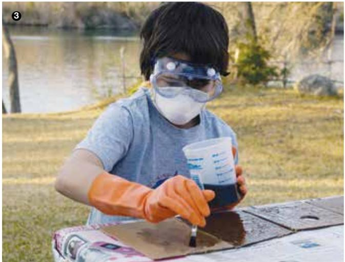
**Step 3**—Using the paintbrush, lightly coat the outside of the walls with resin.
