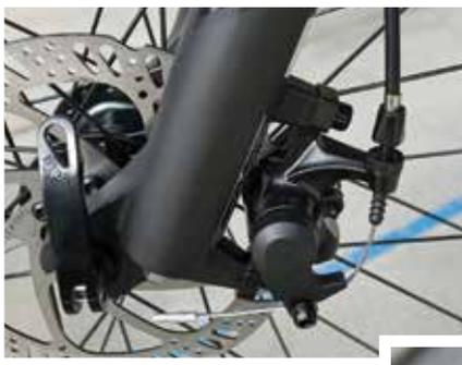
Barrel adjuster on cable disc brake
