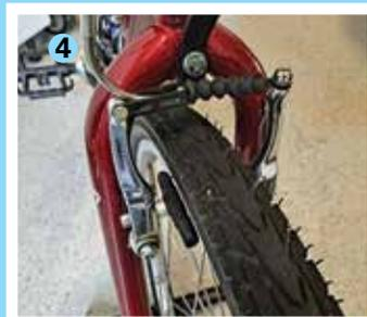
**4.** There should be an equal space between the rim and pads on each side.
