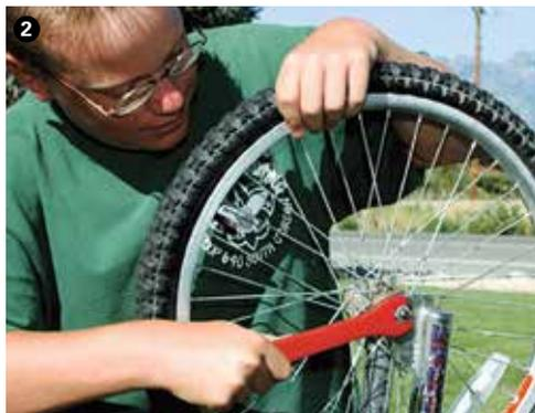
**Step 2**—If the flat is on the rear wheel, turn the crank by hand and shift to the smallest cog on both the rear sprockets and the chainring. Deflate the tire completely, release the brakes if possible, and remove the wheel from the bike.
