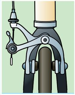
Loosen the anchor bolt or quick release (shown here). On side-pull brakes, this bolt is on the arm. On center-pull brakes, this bolt is on the bridge-wire hook. The main brake cable is now free to move, and you can adjust the brake pads so that they are aligned with the side of the rim when moved against the rim.
