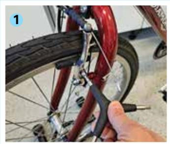
**1.** Align the brake pads and loosen the mounting bolt.
