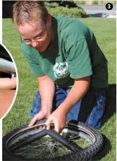
**Step 4**—Inflate the problem tube with enough air that you can find any holes by feeling or hearing the air escape. Dunking the tube in water may help detect holes that are otherwise difficult to locate. Check the corresponding section of the tire for a sharp object that might have caused the flat. Be absolutely sure the object is gone before you continue.
