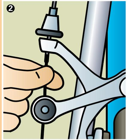
1. To adjust your brake cable, loosen the main anchor bolt. Squeeze the brake lever; unscrew the barrel adjuster. This frees the cable for loosening or tightening to decrease or increase cable tension.
