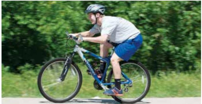
**The quick stop is nothing more than a maximum-effort stop without skidding either wheel. You get a gain in braking efficiency when you shift your hips back on the saddle, or even slide off the saddle and place your stomach on the seat. This transfers more of your body weight to the rear wheel and increases its traction.**
