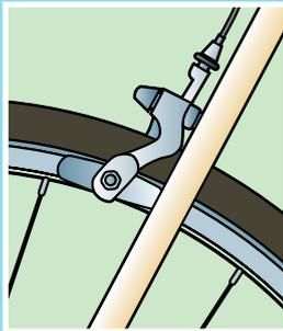
The front edge of the brake pad should be “toed in” so it contacts the rim slightly before the rear edge. Gently bend the flat surfaces of side-pull brake arms, or adjust the washers on center-pull brakes. Once the brakes are aligned with the rim, have a friend hold the brake pads (or use a tool or a piece of string), then tighten their bolts to secure them. You also do this to fix squeaky brakes.
