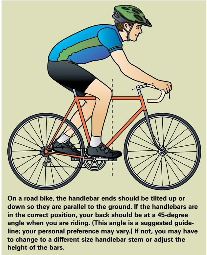
**On a road bike, the handlebar ends should be tilted up or down so they are parallel to the ground. If the handlebars are in the correct position, your back should be at a 45-degree angle when you are riding. (This angle is a suggested guideline; your personal preference may vary.) If not, you may have to change to a different size handlebar stem or adjust the height of the bars.**
