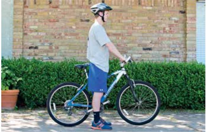
**Check the fit by straddling the top tube and lifting the handlebars until the top tube reaches your crotch. On a road bike with a horizontal top tube, there should be 1 inch of clearance; for a road bike with a sloping top tube, look for 2 or more inches of clearance. For a mountain bike, there should be 2 to 4 inches of clearance.**
