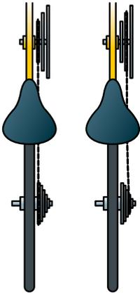
**When approaching a hill, shift the front derailleur to a smaller ring (in which it is easier to pedal) and shift the rear derailleur to a larger gear. For downhill, shift the front derailleur to a larger ring and the rear derailleur to a smaller gear. Avoid cross-chaining; that is, selecting a large ring in the front and a large gear in the back or a small ring in the front and small gear in the back.**
