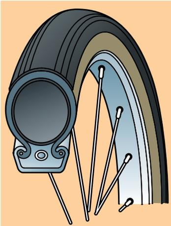
**In a clincher tire, the inflated tube presses the wire-embedded edge, or bead, of the tire casing outward, holding it secure against the wheel.**
