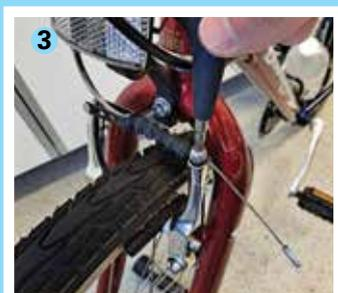
**3.** Loosen the cable pinch bolt. Pull the cable to move the brake arms together until the pads are almost touching the rim. Tighten the pinch bolt.
