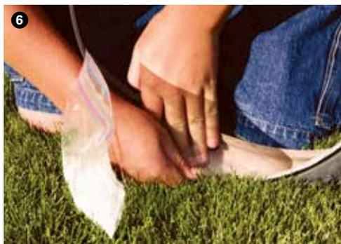
**Step 6**—To make remounting the tire easier, use talcum powder to coat the inside of the tire, the bead of the casing, and the tube.
