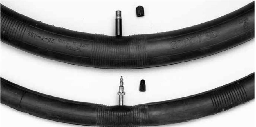
The Presta valve tube, *bottom*, is most often used on narrow rims because it requires a smaller valve opening, which is the rim's weakest point.
