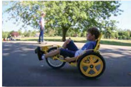
**A recumbent bicycle or tricycle may be easier for a physically challenged person to power. Some are adapted so that they can be pedaled with the hands rather than the feet.**
