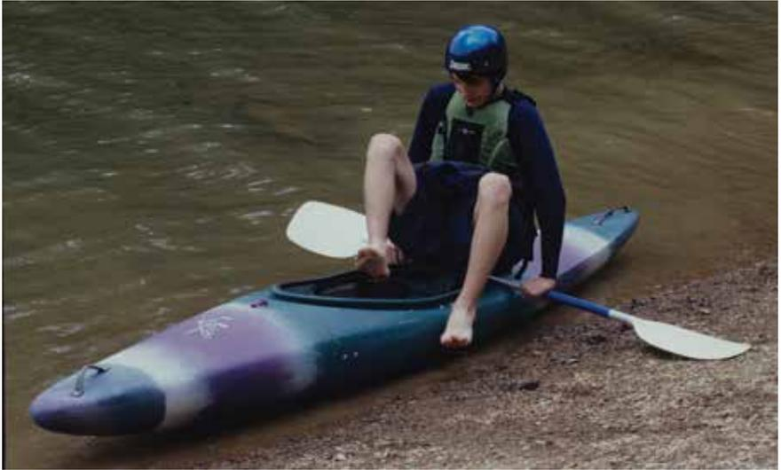
Coaming is the raised edging around the cockpit for keeping water out.
