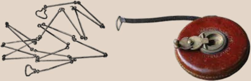
**A Gunter's chain measured the wilderness of the United States. Chainmen laid out the chain and pulled on the handles to measure 66 feet.**
