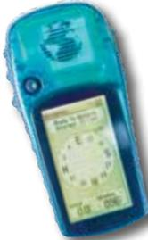
GPS equipment quickly is becoming a more economical and affordable method for measuring distances, and it is simpler to use than the expensive and delicate total station. However, its use is limited because a GPS receiver cannot receive data when something stands between the receiver and the satellites. Surveying using GPS will not work indoors or under trees.
