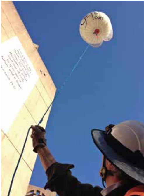
A balloon flies past a new skyscraper, carrying a camera to help evaluate the energy efficiency of the building.
