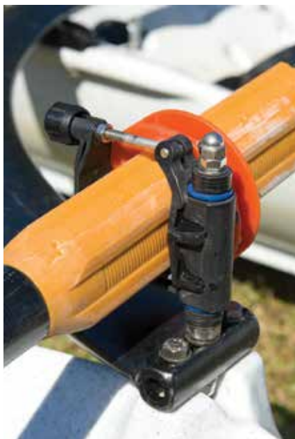
Sleeve and collar in gated oarlock
