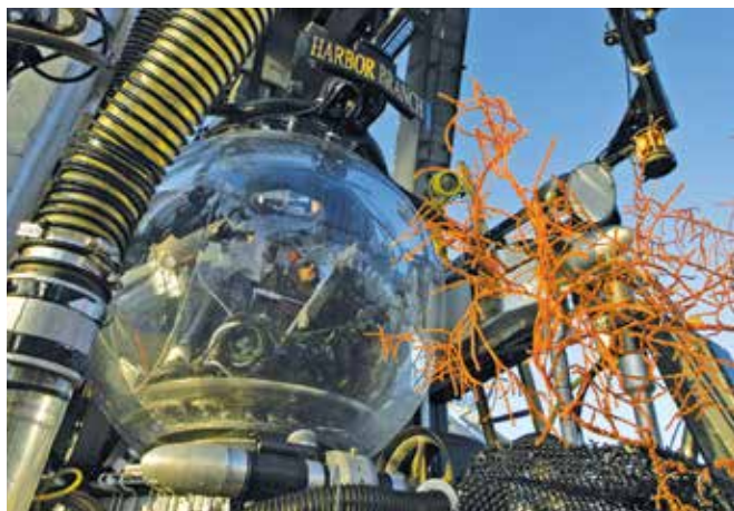
The Johnson Sea-Link is equipped with a variety of tools that scientists use to collect samples from the ocean depths.
