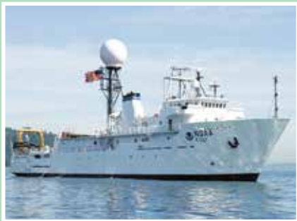
NOAA's Okeanos Explorer is the first U.S. ship devoted to ocean exploration. Commissioned in 2008, this ship is equipped with remotely operated vehicles to investigate areas of interest and has a sophisticated satellite system to allow communication and interaction with researchers on land.
