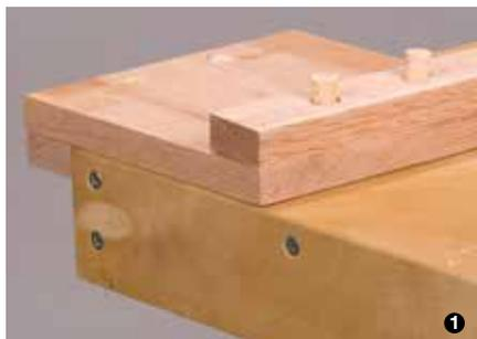
18. Clamp each strip to the base while the glue is drying. Allow the glue to dry completely before removing the clamps. (The photo shows only one strip in place.)
