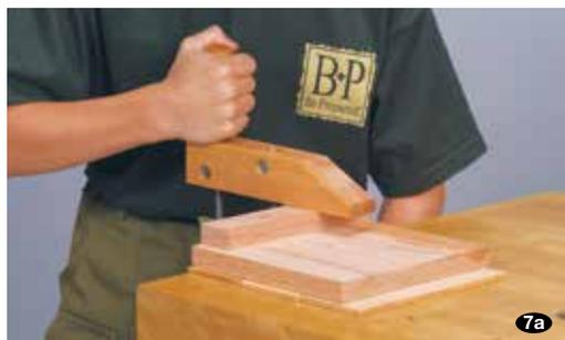
7. Clamp the stacked pieces (7a) to your workbench (being sure to sandwich scrap wood between the base and the bench to protect your work surface). As you tighten the clamp, keep the base and strip properly aligned, with their ends and edges flush. Then use your brace and  $\frac{3}{8}$ " bit to carefully drill each hole (7b). Drill completely through the strip *and* through the base, into the scrap wood beneath.
