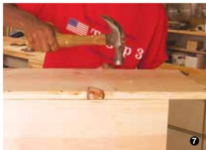
7. Begin assembling the box by nailing the right side to the back panel. Nail through the back into the side piece.
