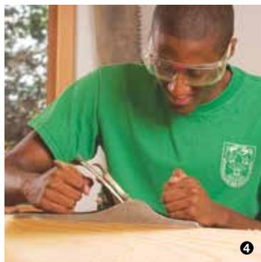
Sawing and planing to the pencil line will give you a 4"-wide board with straight edges.
