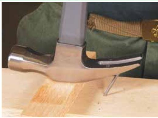
wood under the hammer's head if you need to raise the hammer high enough for the claws to catch the nail head. Then pull back on the handle to pull the nail from the wood.
