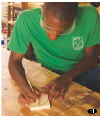
11. Pencil a curved line on each side piece, starting above the hole and rounding to the upper edge, as shown in the drawing. Use a compass or the lip of a cup to guide your pencil.
