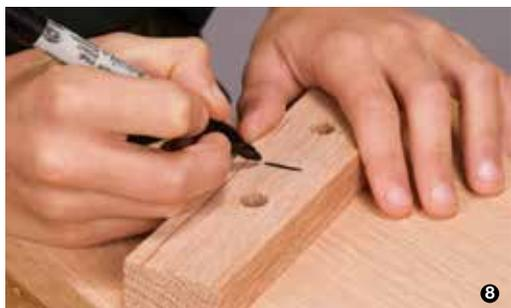
9. Repeat steps 6 and 7, drilling through strip No. 2 and through the base at the opposite edge of the base.
