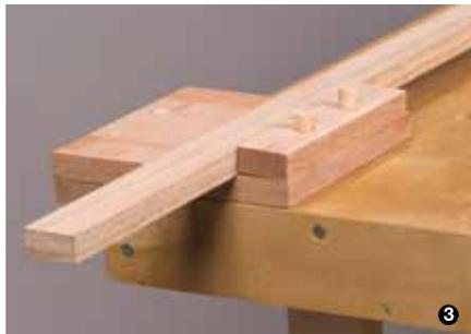
1. Put the bench hook on your work table so that strip No. 2 (the front strip) hooks over the table's front edge.
