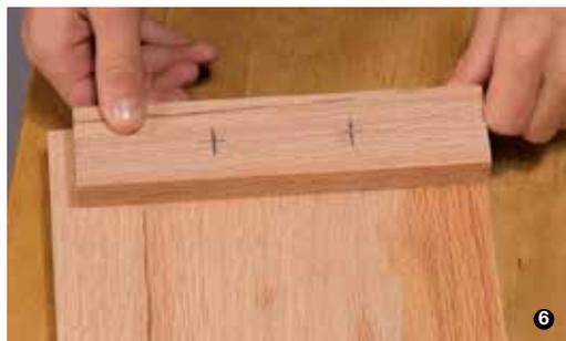
6. Lay a strip on the face of the 8" base piece. Align the strip's edge and one end flush with the base's edge and end, as shown.
