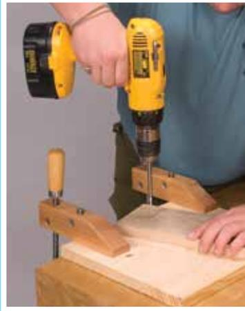
To start a hole, push the point of a nail into the wood to make a small dent. The dent will help keep the drill bit from skittering across the wood as you begin drilling. Put a thick piece of scrap wood under the drilling area to prevent damage to your workbench or table, in case the
