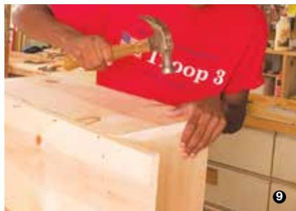
9. Attach the left side, nailing through the back panel into the side piece and through the left side into the floor.
