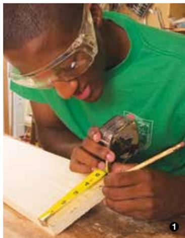
1. Measuring from the straight and square edge of the 1" x 6" board, mark a width of 4" near each end of the board.
