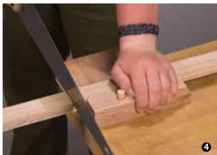
4. Using the heel of your free hand, push the board tightly against the bench hook's back strip as you use your other hand to saw. Your bench hook will help you hold the board much steadier than you could hold it by hand alone.
