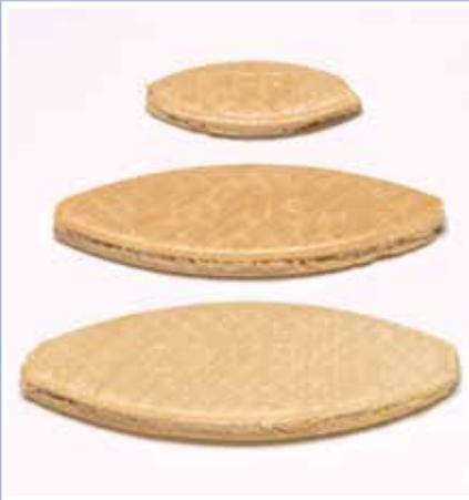
A new approach to the traditional technique of the dowel joint is called *biscuit (or plate) joinery*. "Biscuits" are essentially flat dowels: thin, football-shaped pieces of compressed beechwood that are glued into slots much as dowels are glued into holes. A special machine called a biscuit (or plate) joiner cuts a crescent-shaped slot in each of the pieces that are to be joined. The slots can also be made using a router with a biscuit-cutter bit.
