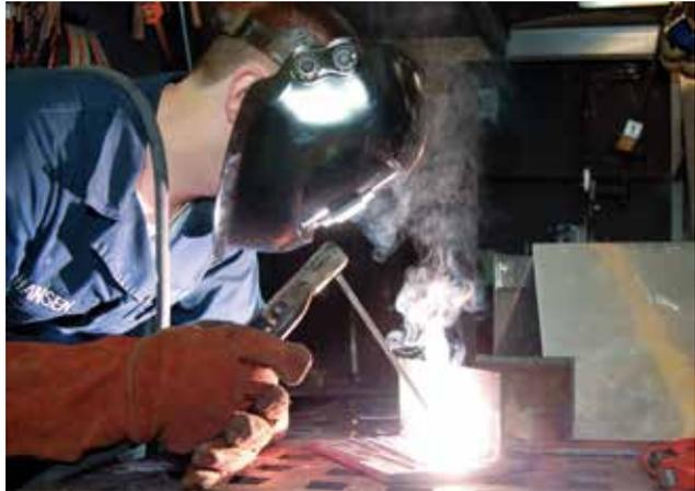
**Welding beads with shielded metal arc welding**
