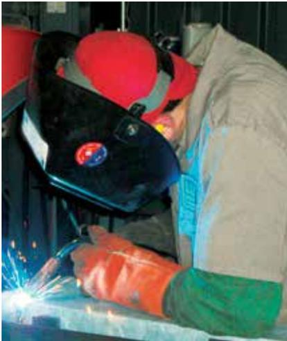
**Gas metal arc fillet weld**
