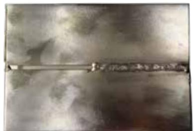
**Tack holds weld in place as weld progresses**
