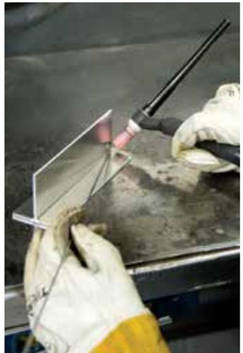
*A fillet weld is a right triangular-shaped weld formed at the interface between the vertical and horizontal members of a T-joint. A double fillet weld is a T-joint with a fillet weld on both sides of the vertical member of the joint.*
