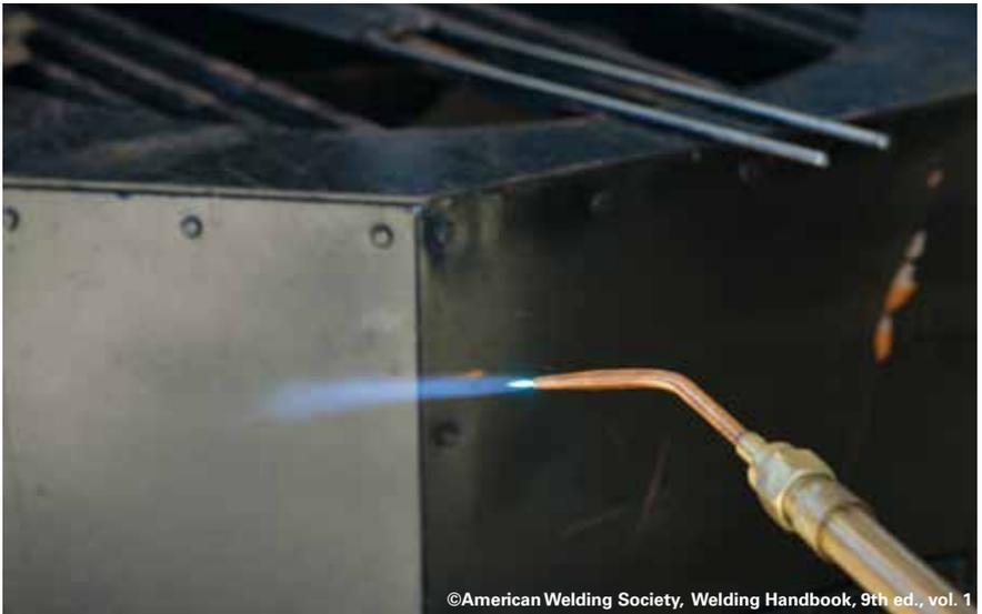
Oxy-fuel welding is one of the simplest methods of joining metals and has been used for more than a century.
