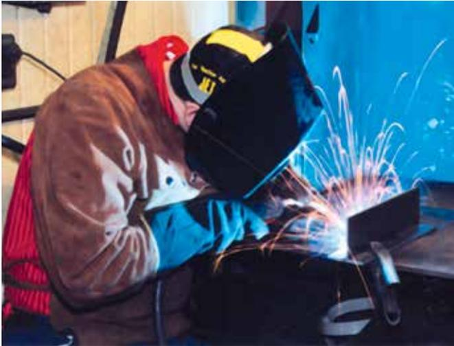
**A fully protected welder wears the proper clothing along with a welding helmet, safety glasses with side shields, leather sleeves, leather gloves, and leather shoes or leather boots. Wearing protective leather clothing minimizes the risk of fire and burns from spatter. Store leather garments in a well-ventilated area.**
