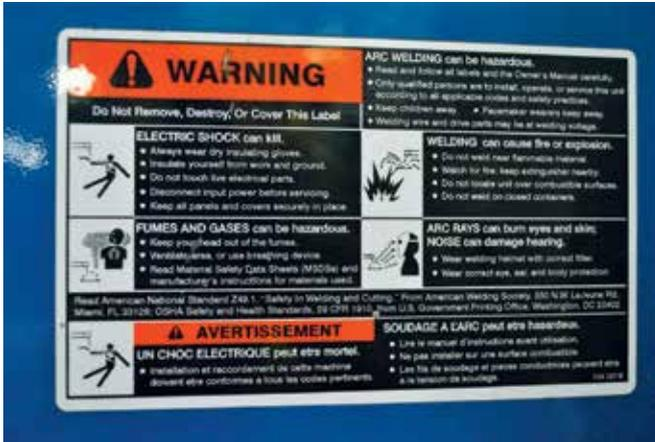
Always read all warning labels on arc welding components and filler metals container.
