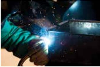
**Step 9**—Place a  $\frac{1}{2}$ " long fillet weld in each corner to keep the popcorn oil from leaking. Full-length welds are not necessary. You can clamp thicker metal to the outside to absorb excess heat if you have trouble with burn-through.
