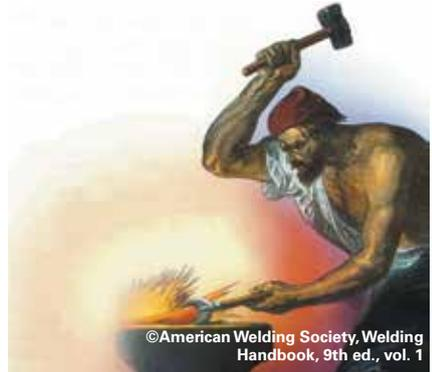
**forge welding.** A welding process in which two or more pieces of metal are heated, then hammered together. Used since ancient times, it is one of the simplest methods of joining metals.
