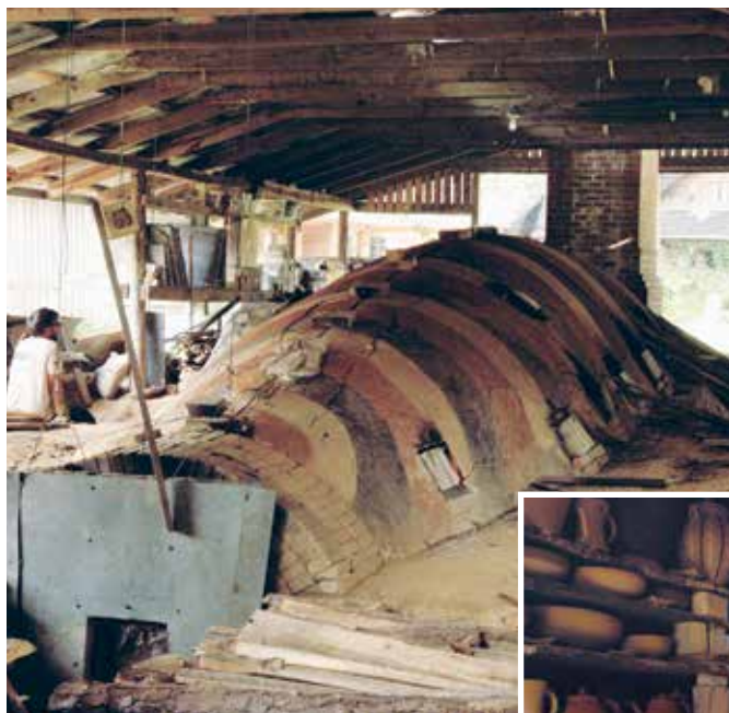
Mark Hewitt's 900-cubic-foot kiln was modeled after a 14th century kiln from northern Thailand.
