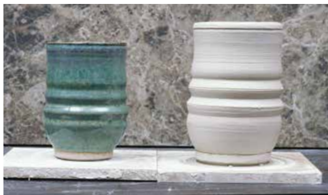
The fired piece at left shows the effects of shrinkage when compared with an identical piece, right , that has not yet been fired.
