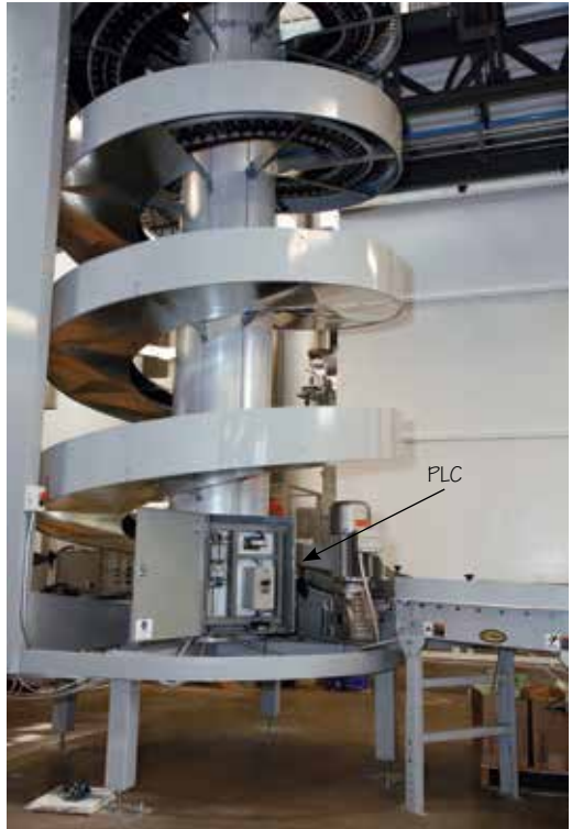
This PLC controls motors and sensors in an automated distribution facility, including this spiral conveyor system.
