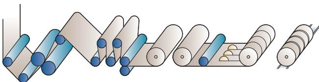
**All Rolled Up.** The paper passes through a calender stack that gives it a smooth and even surface. Then it's collected on a large reel in jumbo rolls that weigh 40 tons or more. On the winder, the rolls are slit to desired widths and wound on cores, ready to be shipped to customers or cut into smaller sheets.
