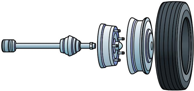
**An exploded view shows the individual parts separated from one another but still in their correct relative positions.**
