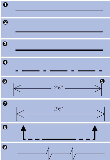
6. **Dimension line.** Thin line with arrow points touching the extension line and with a break in the middle for the dimension numeral (in a mechanical drawing), or
