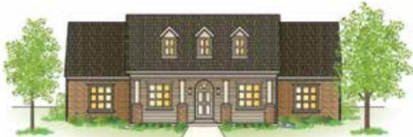
**Items like the depth of the foundation, type of roof, and height from the ground are all shown in elevation drawings.**
