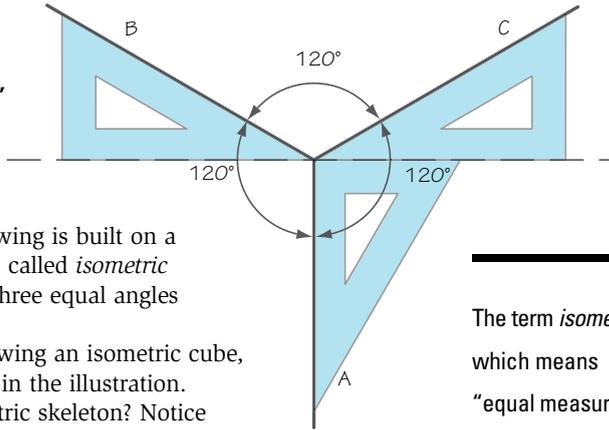
An isometric drawing is built on a skeleton of three lines called *isometric axes*. The lines form three equal angles of 120 degrees each.
