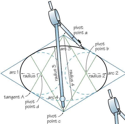
At these points, draw perpendicular lines to the sides of the isometric square, using a 60-degree triangle. The four intersections of the perpendicular lines (*a*, *b*, *c*, and *d*) will be the center from which four arcs can be drawn with a compass to complete the isometric circle.
