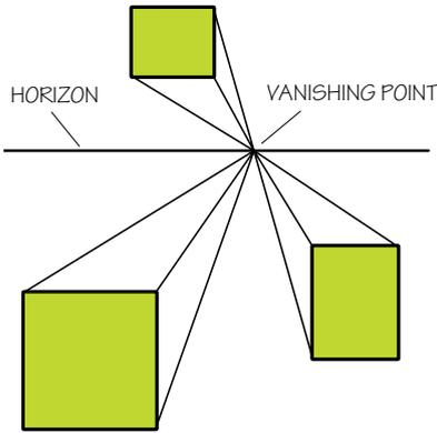
**In a perspective drawing, the far-off parts look smaller and closer together than the nearby parts.**
