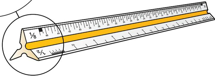
A special ruler used to measure or draw a scale drawing is called an *architect's scale*. This ruler divides dimensions for you, simplifying the process of measuring or drawing objects that are larger than the paper or smaller than you want them shown. By comparison, an *engineer's scale* is more detailed and shows fractions up to sixtieths of an inch.
